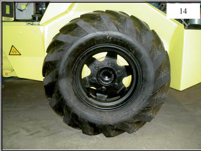
Check air pressure in rubber tyres (3,5 bar)
