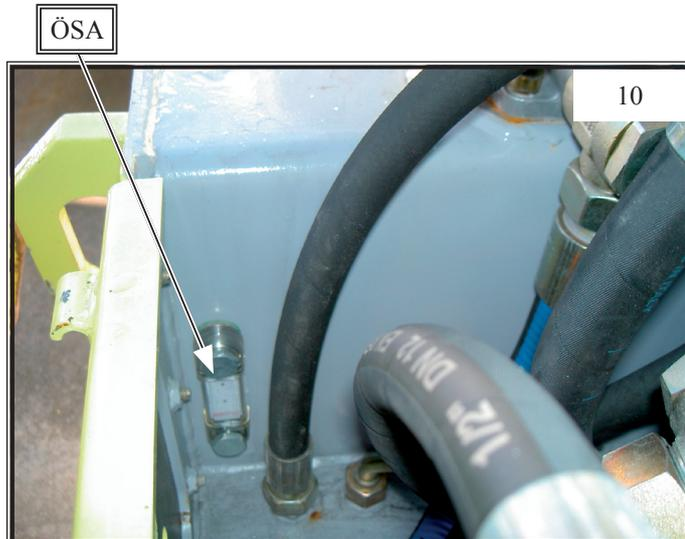
Check hydraulic oil level and top up if necessary
