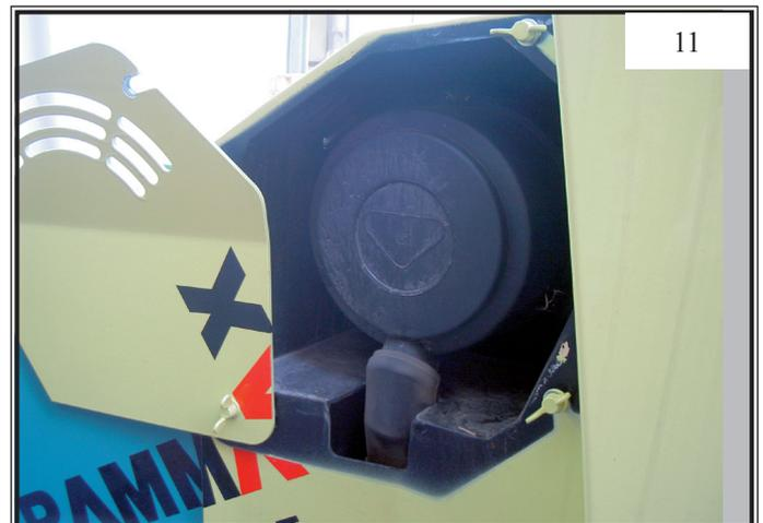
Check soiling of the air filter
