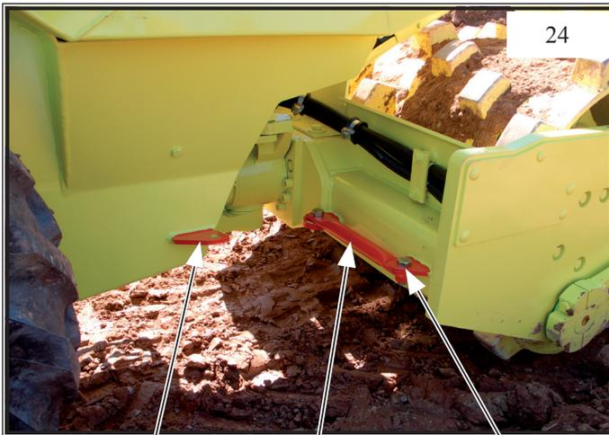
After driving the machine onto a suitable transport medium, the hex bolt „K“ must be dismantled, the transport safeguard „T“ must be turned into the support „BL“ and safed with the hex bolt „K“. (Bild 24)
