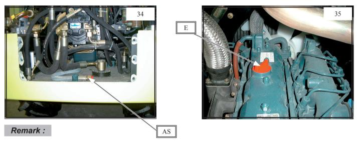
Only drain off the engine oil when the engine is warm. For exchange intervals for engine oil, see the Kubota V2203 manual (Annex)
