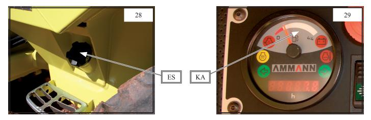
Contaminated fuel can lead to the failure of or damage to the engine. If necessary, top up fuel through a sieve filter. Clean the area surrounding the filling hole and refuel. Fuel: see the operating manual of the Kubota V2203! (Annex)
