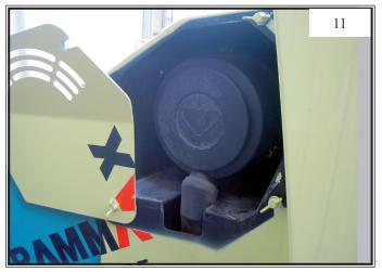
Check soiling of the air filter
