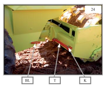
After driving the machine onto a suitable transport medium, the hex bolt "K" must be dismounted, the transport safeguard "T" must be turned into the support "BL" and safed with the hex bolt "K". (Bild 24)
