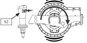
The vibration of the machine is activated by the 3-position-switch of the driving lever. By turning the switch to the right, seen from the driver's seat, the vibration forward is activated (position 1). By turning it to the left, the vibration backward is activated (position 2). The middle position of the switch is for de-activating the vibration
