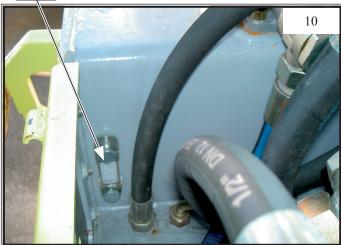
Check hydraulic oil level and top up if necessary
